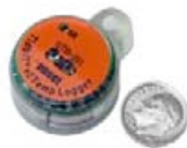
Figure 2: Photograph of a logger similar to that used on Reservoir Creek (the coin is equivalent to a 10 cent piece)
