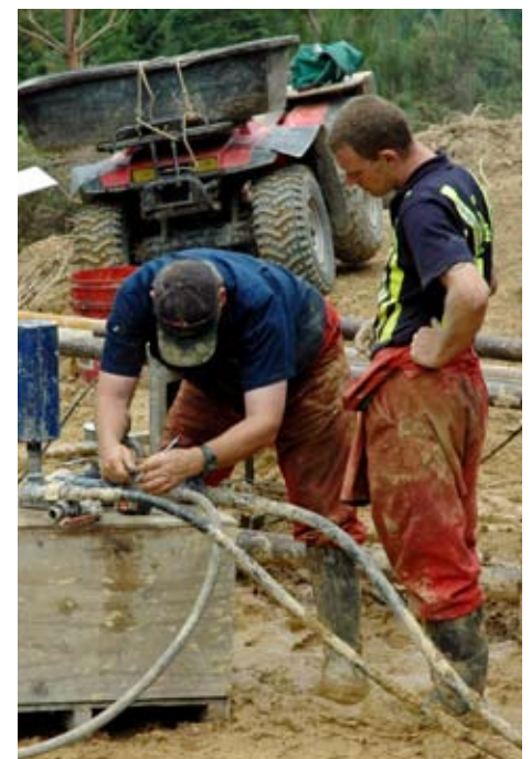
Drillers pressure testing rock core samples.
