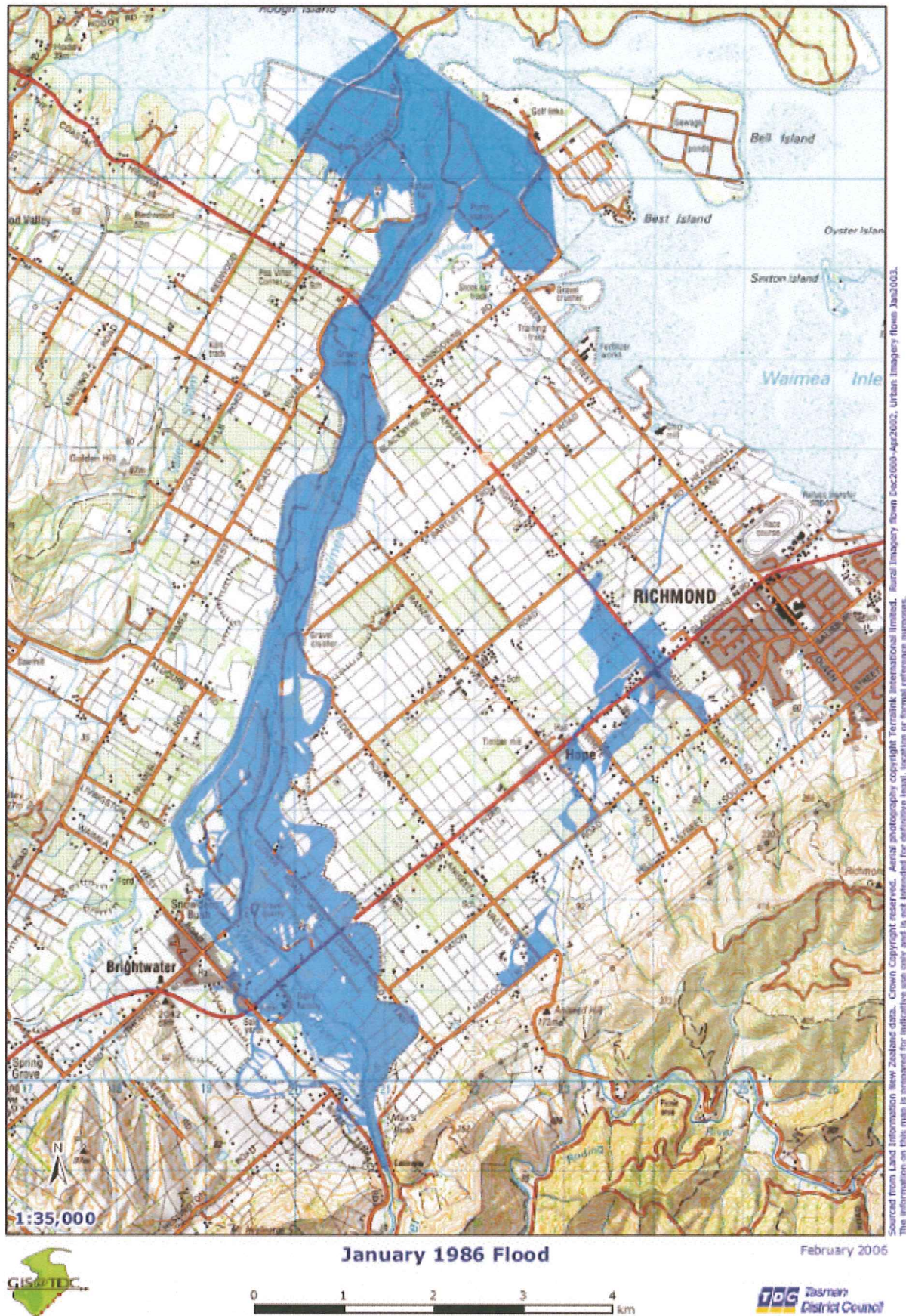
Figure 4.6 Extent of Inundation in the January 1986 Flood (Estimated by TDC)
