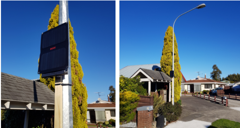
Photo 7: An example of the outdoor dust information nodes (ODINs)
