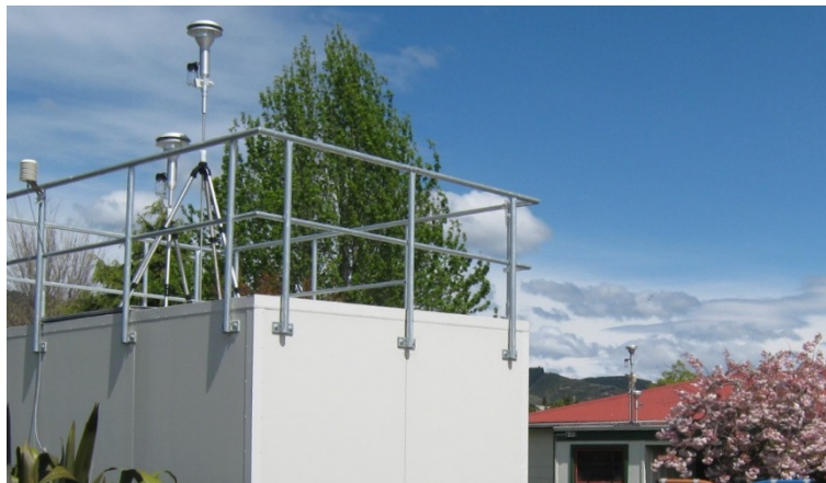
Photo 1: Richmond Particulate Monitoring instruments 2019 showing new portacom and BAM 5028 in foreground and old FH62 BAM and Partisol in background.
