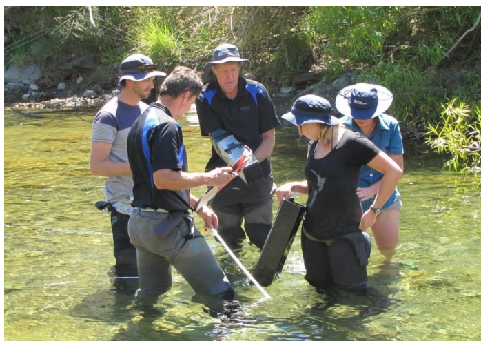
Monitoring staff at a training and quality control exercise. Here comparing black disc water clarity measurements to ensure inter-operator accuracy (Jan 2015).
