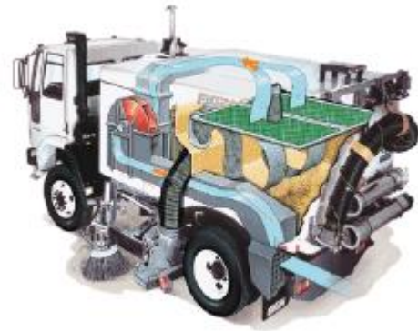
A vacuum sweep vehicle for removing road deposited sediment
