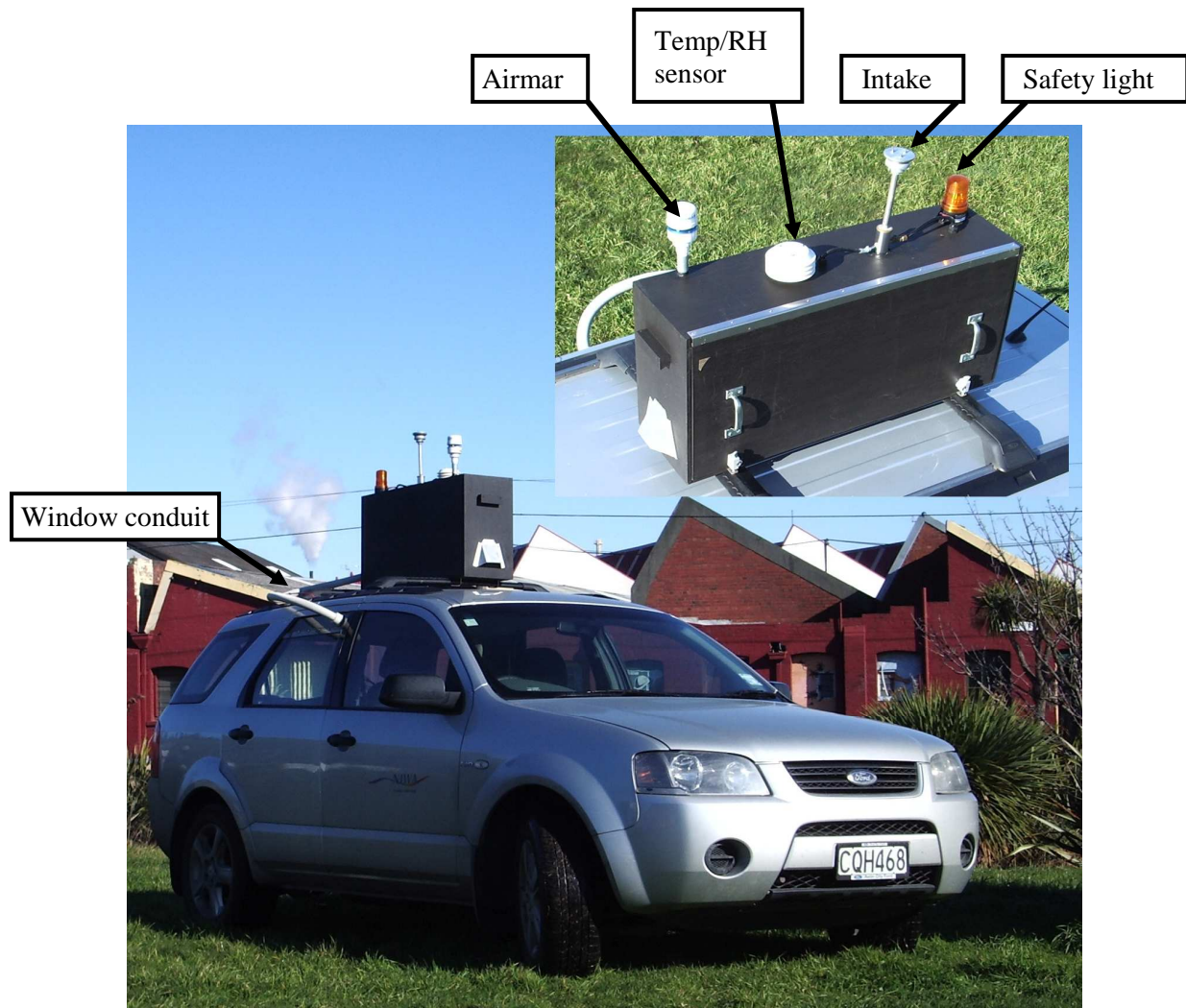
Figure 2-1: Mobile monitoring vehicle and (inset) rooftop enclosure. Rooftop instrumentation (including Airmar and temperature + relative humidity sensor) and air intake is shown.
