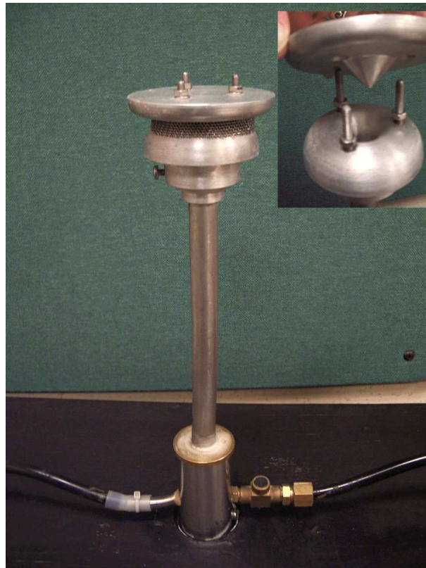
Figure 2-2: Sample tube intake, showing (inset) convex top-piece designed to direct flow into the tube.
