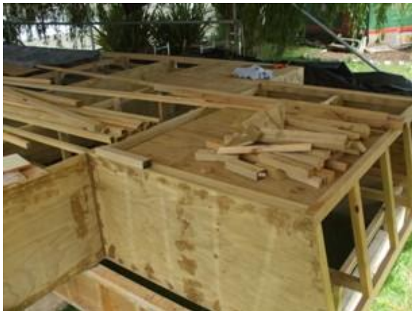
Stern end – recesses for engines each side
