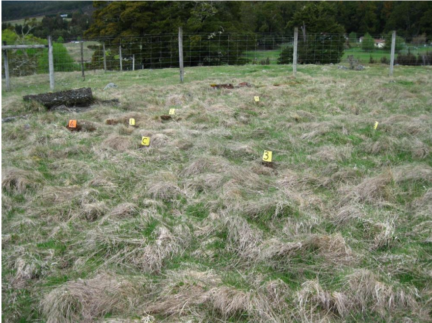
Above: Dip site with 1.4% arsenic near dip entry at flag “4” and flags showing extent out from that end.
