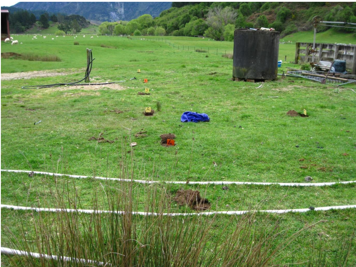
Flags showing extent of arsenic contamination out from the corrugated iron spray dip
