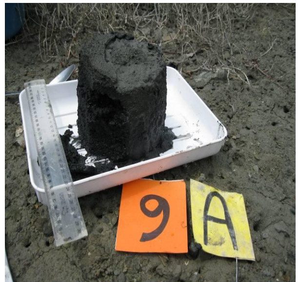
Anoxic core from Dynea culvert
