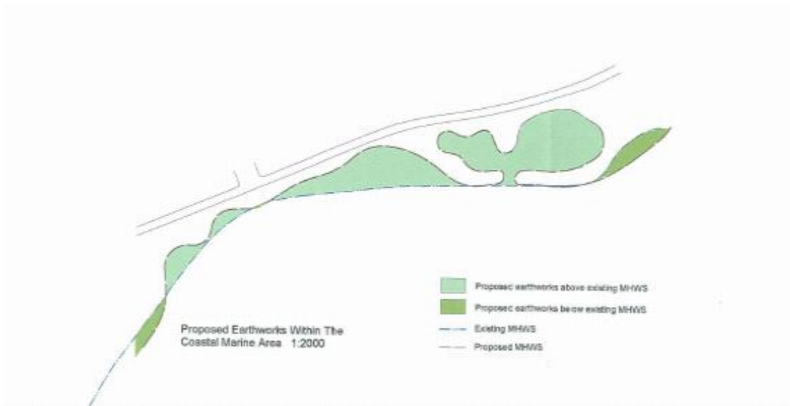
Figure 1: Proposed Earthworks within the Coastal Marine Area
