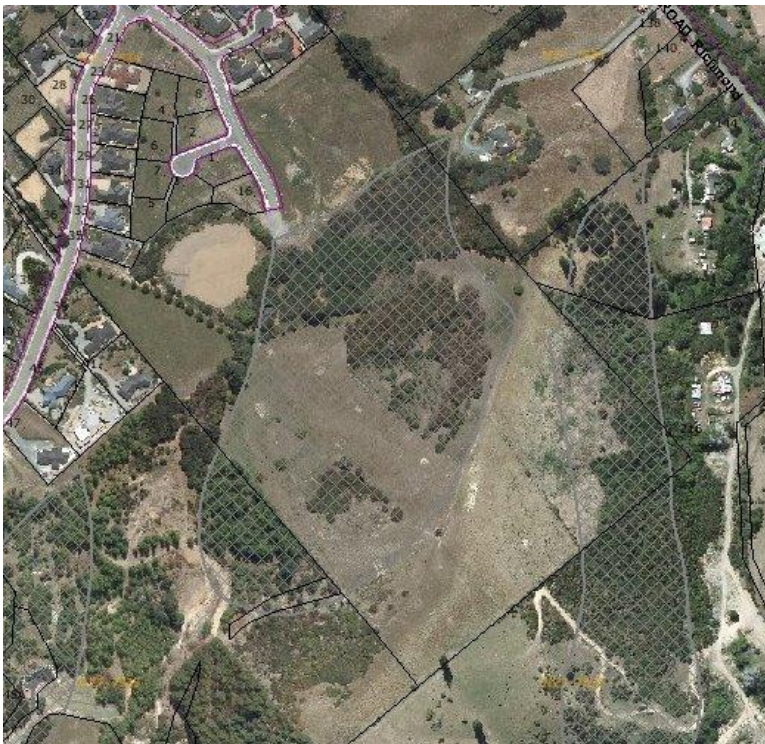
Figure 2 Slope instability risk areas with aerial photo backdrop
