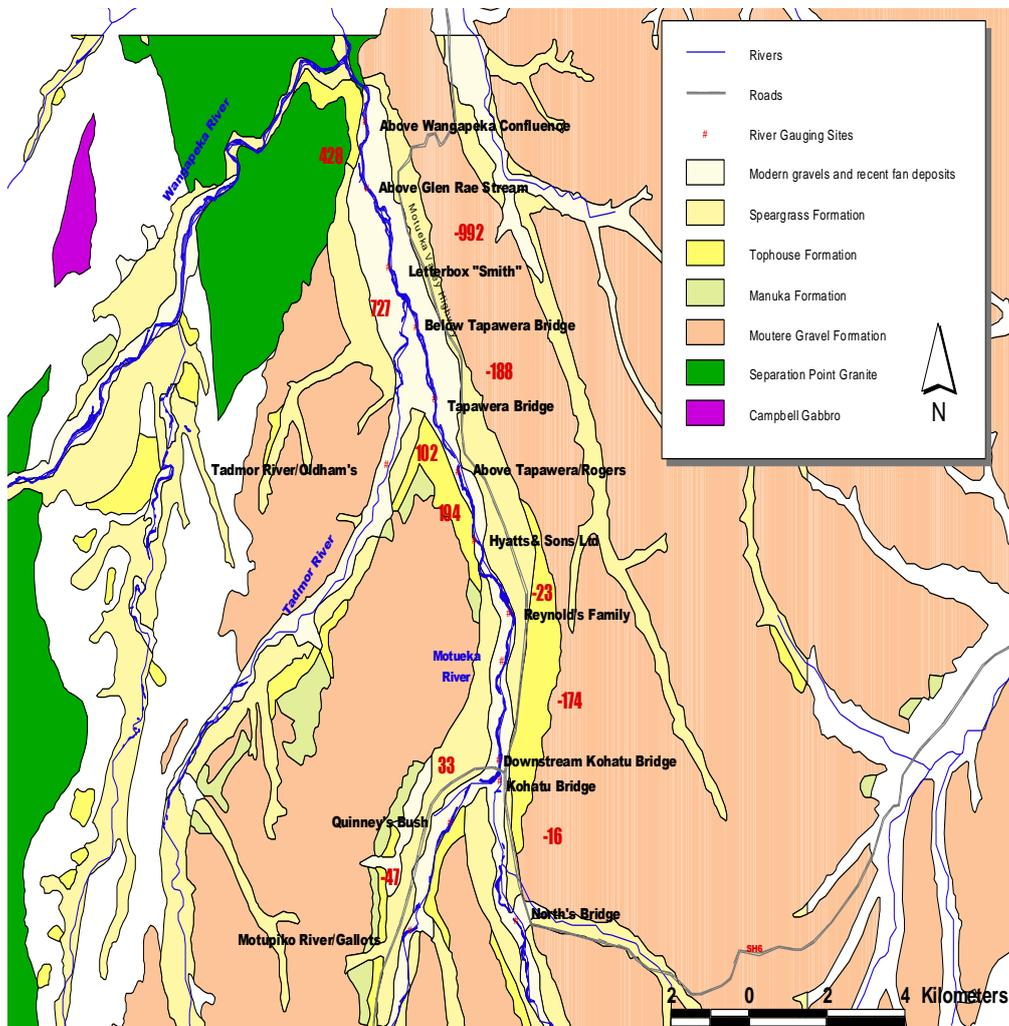
Figure 5: River flow loss and gain from gaugings in February 2002
