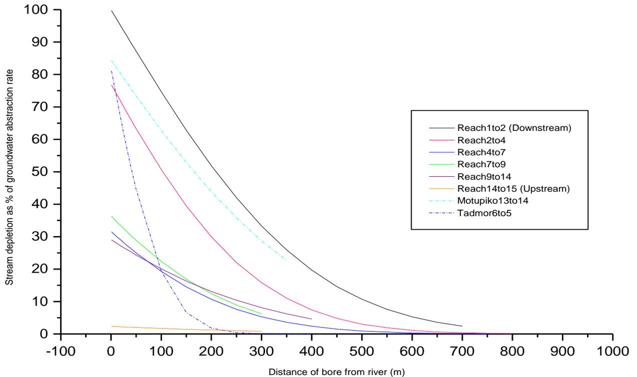
Figure 8: Stream depletion when pumping from within the Modern Gravels
