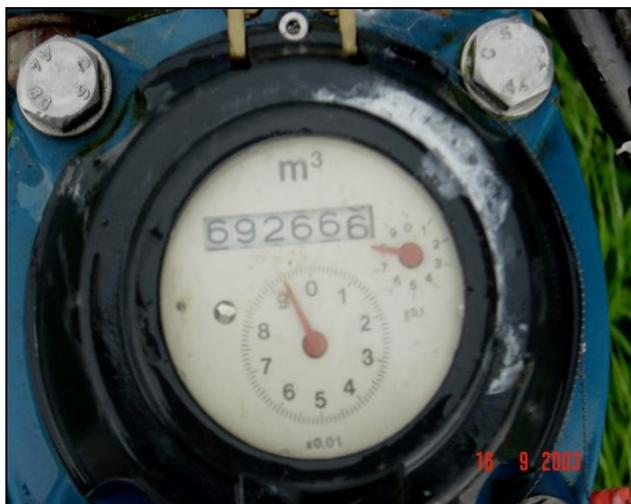
**Figure 3:** An old Style Meinecke Meter. Reading is 692666.
