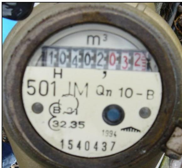
**Figure 1:** A Socam Meter. Reading is 10402
