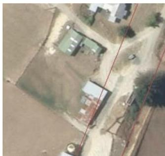
*The example shown is a structure intruding (encroaching) on a Council-owned road (the road boundary is shown as red lines)*
