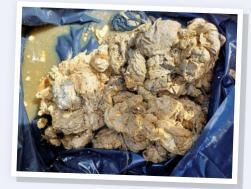
In this case, the blockage was so bad that the contents had to be cleared by hand before a commercial sucker truck was called in to remove the entanglement of wet wipes and sewage.
