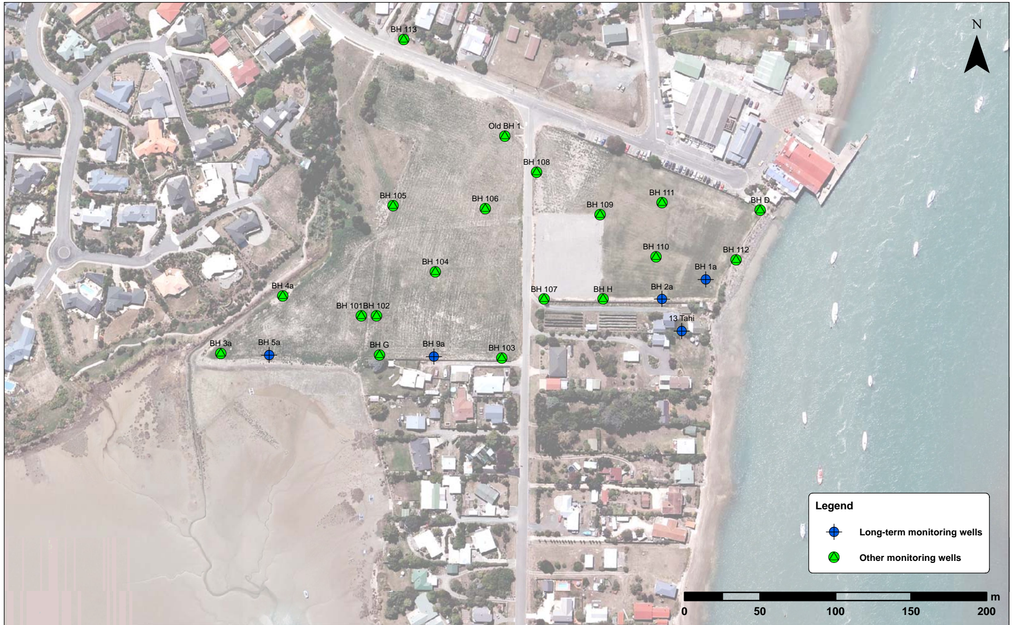
Figure 1 : Groundwater Monitoring Wells
