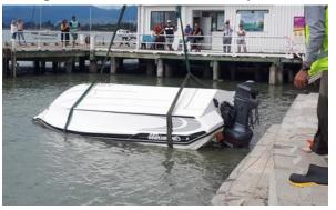
This vessel got swamped when the tide changed from bow on to stern too whilst unattended. Sinking the vessel and rotating her upside down under the floating dock at Mapua.
