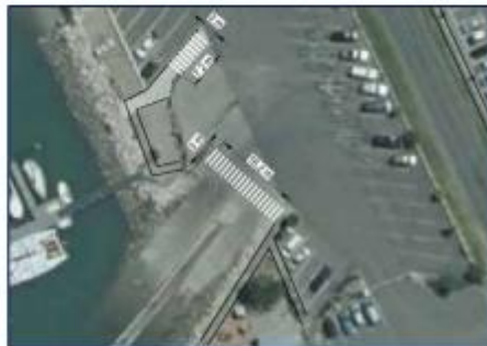
Figure 34: Motueka – Recommended Pedestrian Safety Enhancements (Concept)
