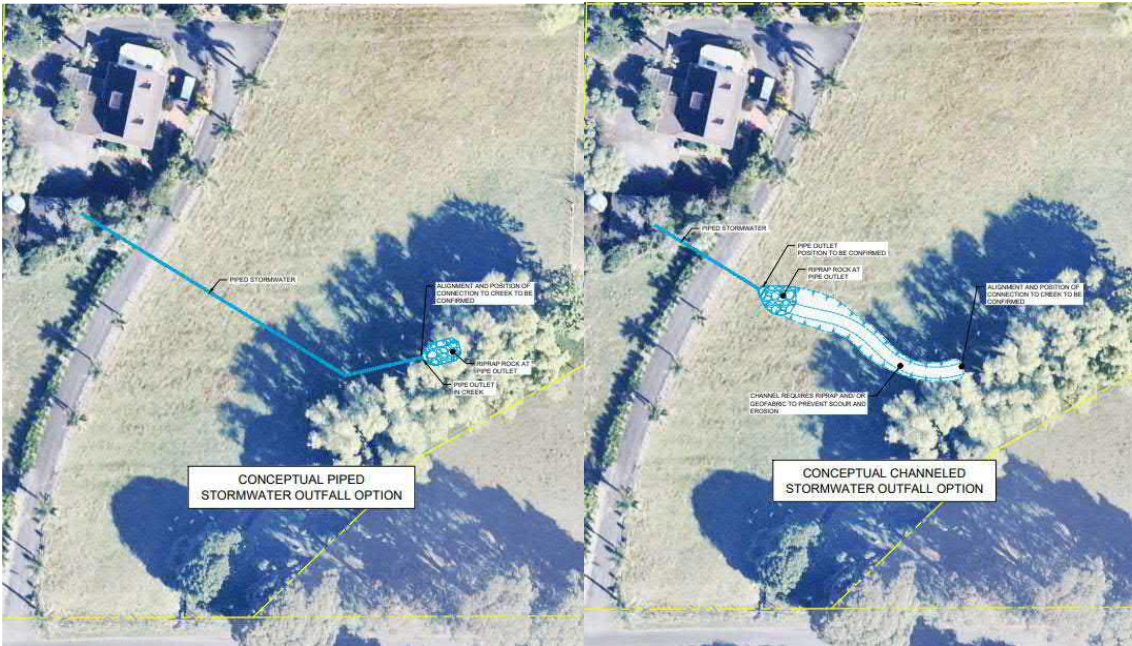
Figure 1 - Conceptual piped stormwater outfall option(L) and conceptual channelled stormwater outfall option (R).
