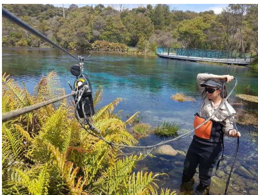
Figure 2-3: Te Waikoropupū instrumentation. (A) Base station showing electronic logger housing, frame, solar panels, AIRMAR weather station, light sensor and telemetry aerial. (B) The instrument water quality package showing the C-Star (with ZebraTech wiper unit fitted) strapped to the EXO-2 sonde (above) with the whole package attached to the flying fox cable with pulleys. (C) Flying fox deployment ready to go. (D) Deployed instrument package sitting in position ready to be lowered beneath spring surface.
