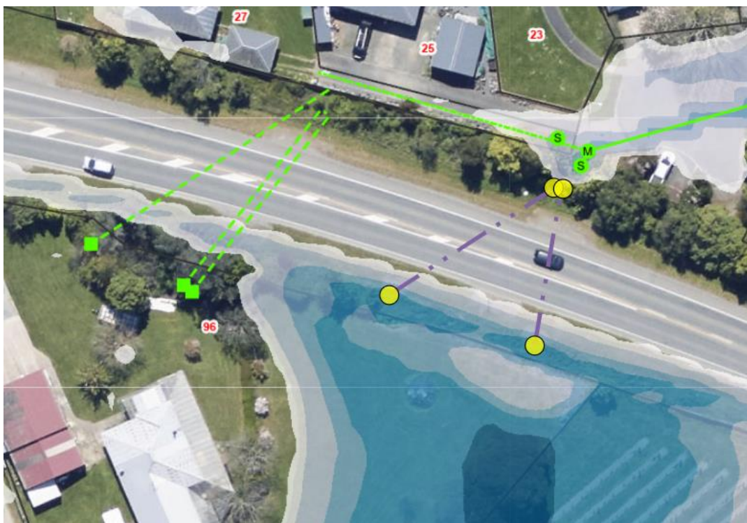
Figure 2.1: Location of newly added culverts shown in purple line (supplied by TDC, 4 September 2024). Rintoul Place properties shown to the north
