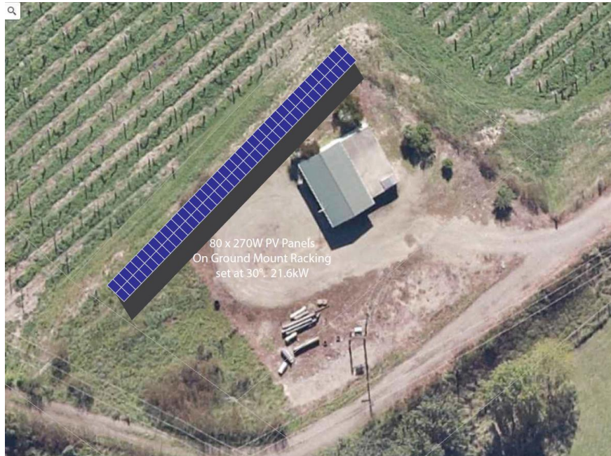
Proposed solar photovoltaic array to power Brightwater water pump station and treatment plant
