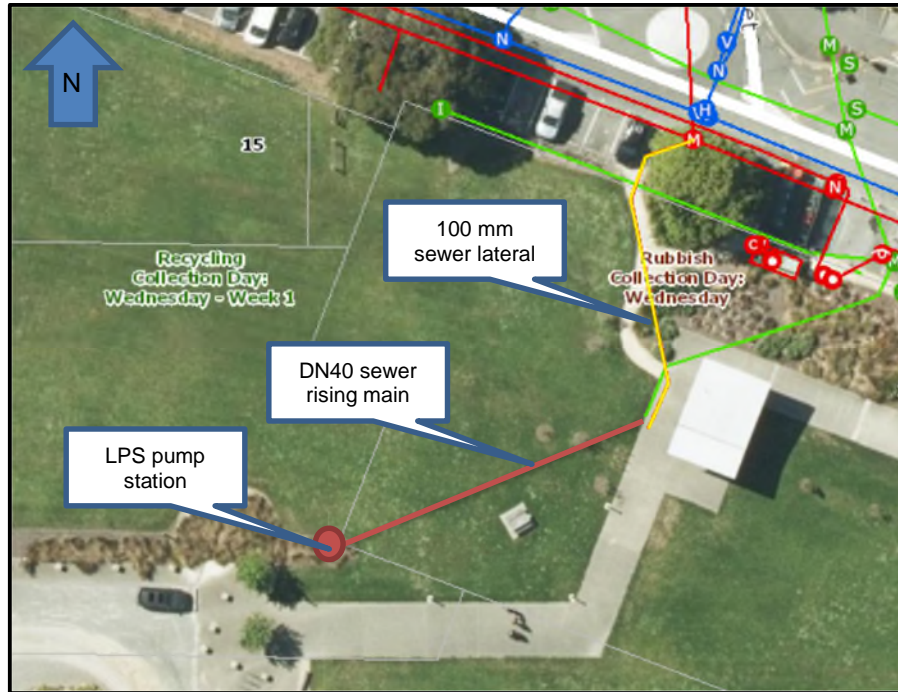
Figure 5: Proposed Sea Scout Building wastewater servicing.
