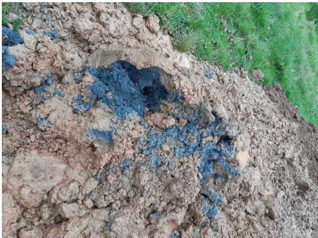
Figure 5. Potentially Liquefiable Blue Silts
