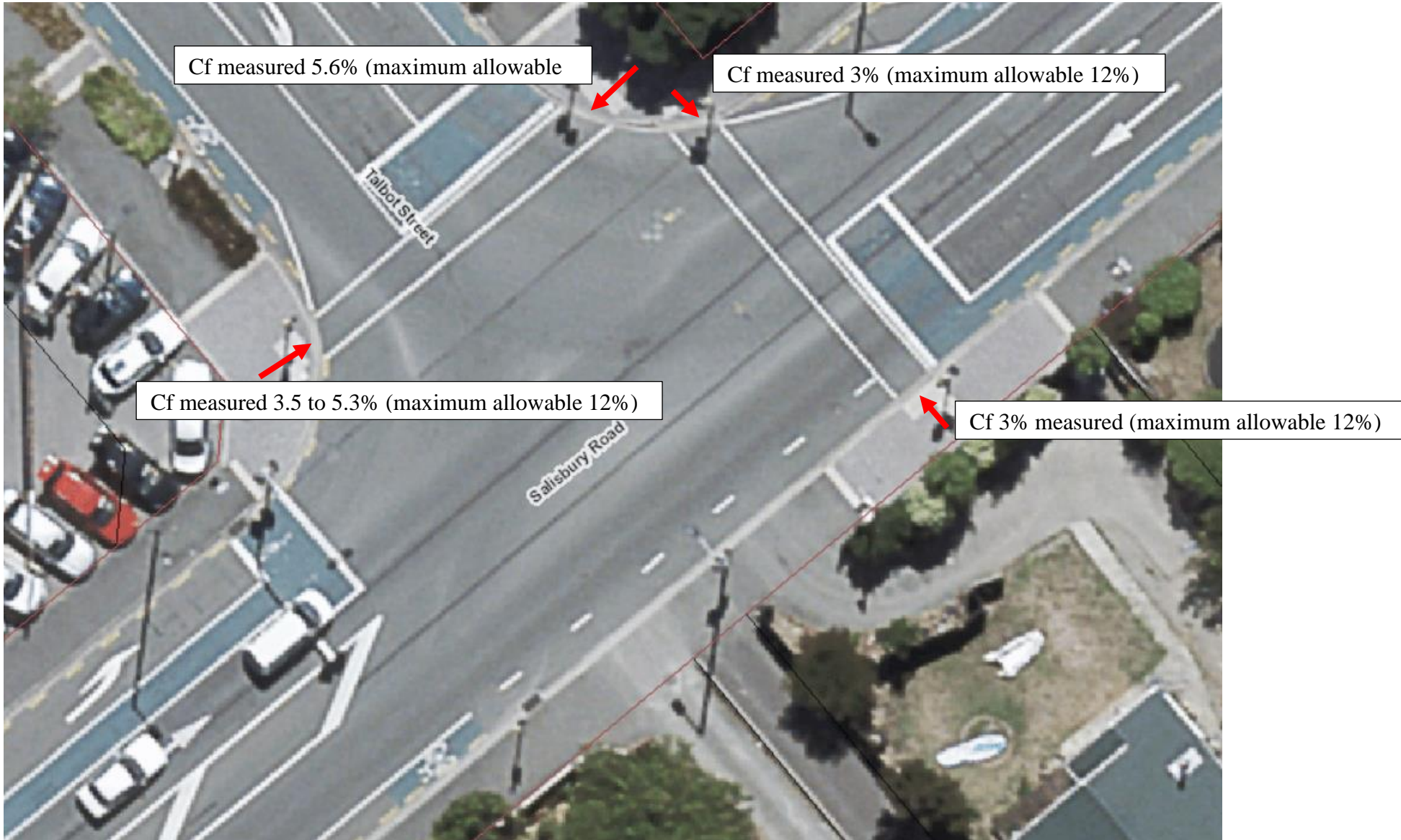
Talbot/Salisbury Rd Pram Ramp Cross falls as measured on site 1/09/17
