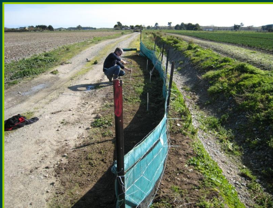
Picture: Field tests of sediment movement on dairy land converted to brassica production in the Horowhenua district
