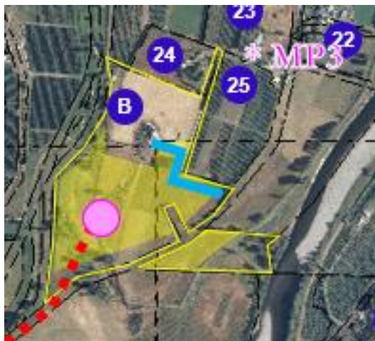
Figure 1: extract from the Acoustic Engineers report showing the 3m high noise mitigation bund. Bund is represented by the Blue line.
