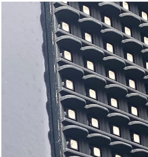
Zoomed in image of LED's and eyebrows LED's are at 10mm centres
