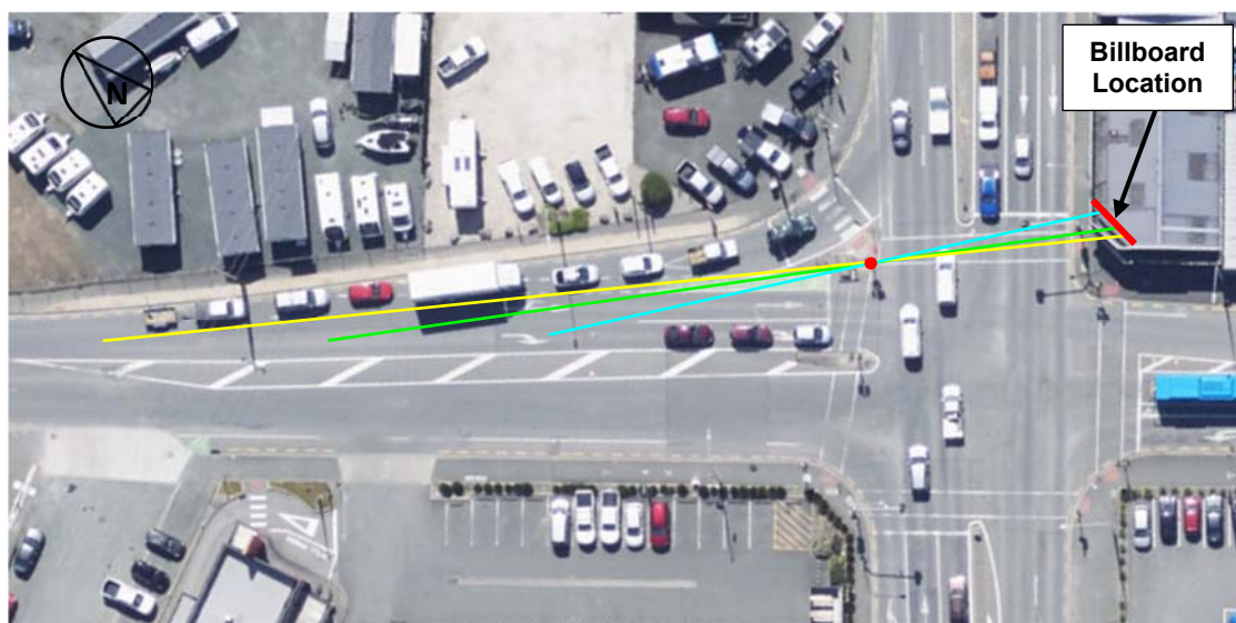
Figure 4: Sightlines Showing the Primary Signal Appears to Move Relative to the Billboard as a Driver Approaches
