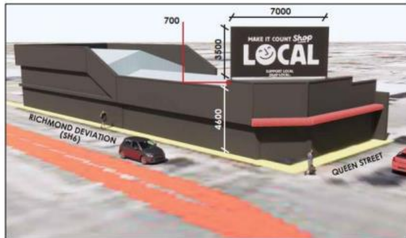
Figure 6 Schematic design of proposed west facing static billboard on top of the PetMart building at 332 Queen Street (DCM Urban)
